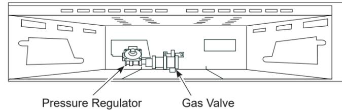
1. Use an adjustable wrench to unscrew the hex-nut cap from the pressure regulator.
