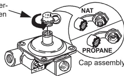
3. Turn the metal cap so the type of gas being converted to is displayed and replace the protective plastic cover. **(Do not over tighten)**
