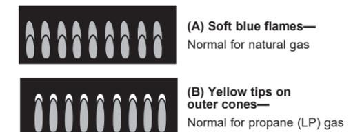
Long, bright yellow flames are not normal. Normal flames may show signs of an orange tint when well heated or signs of flickering orange due to particles in the gas or air.
